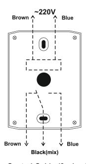
Power Relay Control Cable (3 wires)
