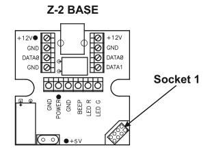
Both Z-5R and Matrix-II K controllers have a symmetric service pin connector for adapter connection via Socket 1.
